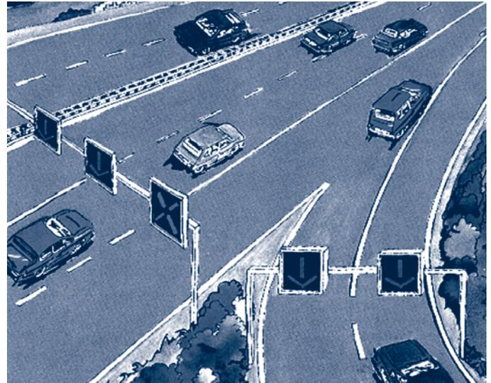
Figure 28. Junction control scheme on German autobahn system.
