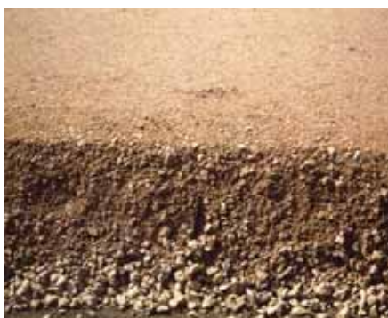
Figure 9.5: Good quality crushed stone is the most common form of roadbase
