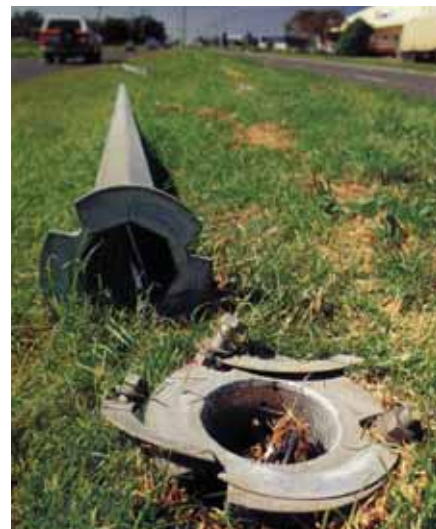
Figure 8.3: Frangible lamp post after vehicle collision, Australia
