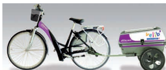
Electrically-assisted bike for maintenance
