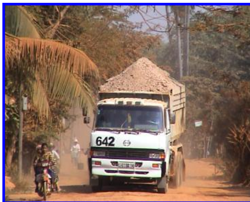
Figure 3 – Truck bodies extended in Cambodia to carry at least 20m 3 of construction materials on 3 axles.
