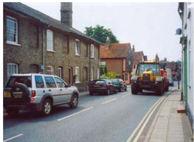
Fig. 3.14 Village speed reduction measure – the provision of on-street parking helps to calm traffic speed.
