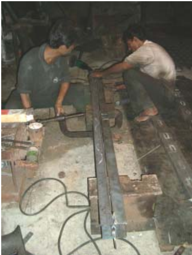
Figure 3.1: Manufacture of Side Panel Members (see Figure B4)
