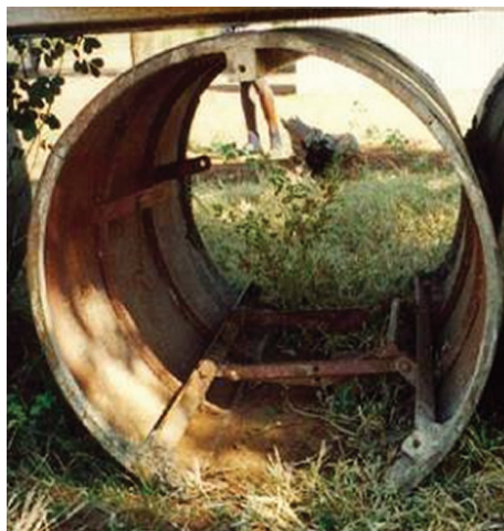
Figure 8.20 Reusable steel mould for cast in situ culvert
