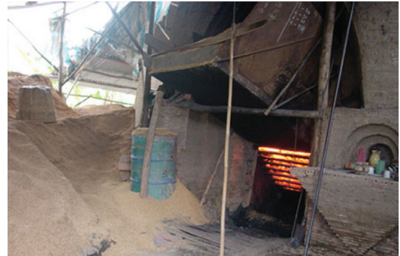
Figure 7.28 - High quality burnt clay bricks produced in small 'beehive' kilns fired by rice husk. Bricks can be fired using coal, wood or other agricultural waste products
