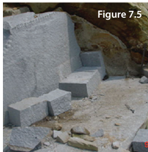
Figure 7.3: Hand dressed stone. Figure 7.4: Hand quarrying of stone. Figure 7.5: Hand quarried granite stone blocks. Figure 7.6: Manual quarry operations can create local employment, however good management is required to ensure a safe working environment.
