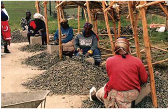
Figure 7.47 Aggregate can be crushed and screened by hand or machine
