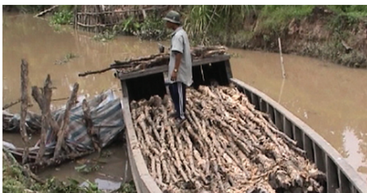
Figure 7.38 Timber poles for piles (not covered by this guideline) for a concrete box culvert in very soft ground
