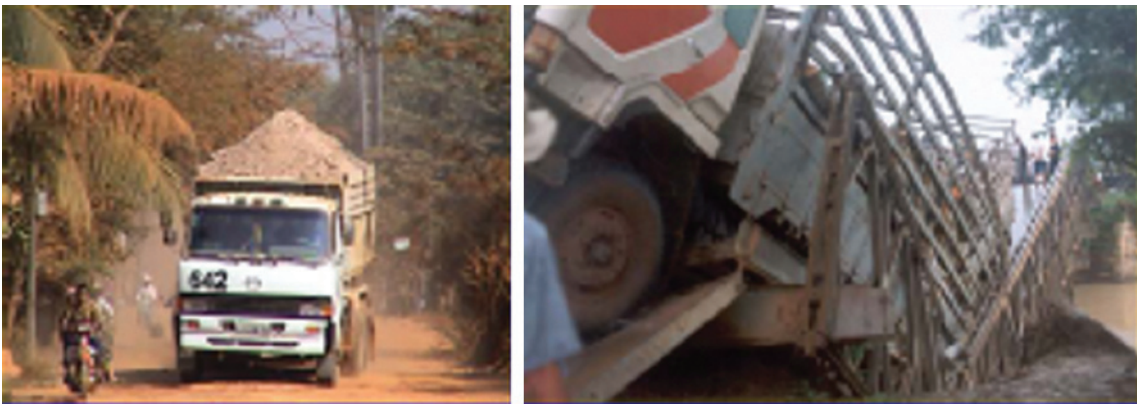
Figure 3.1 Overloading and risk of related structures failure are important considerations for some routes
