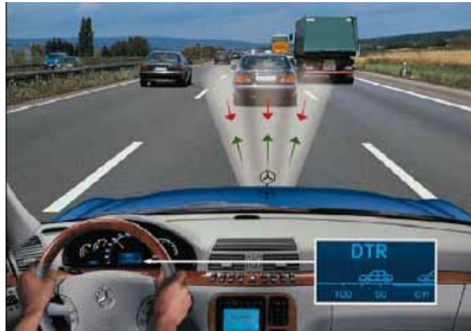
Figure 7.6. Principle of ACC
