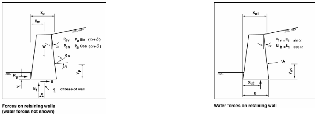
Figure 5-2: Forces acting on a gravity wall
