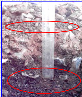
Poor grading and segregation in macadam
