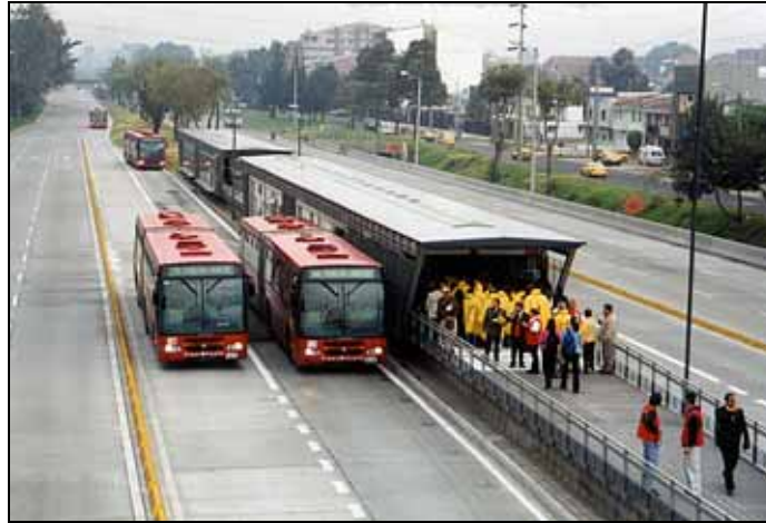
Figure 1 The Bus Rapid Transit (BRT) system in Bogotá (Colombia). Photo by Manfred Breithaupt, GTZ photo CD ( www.sutp.org ).
