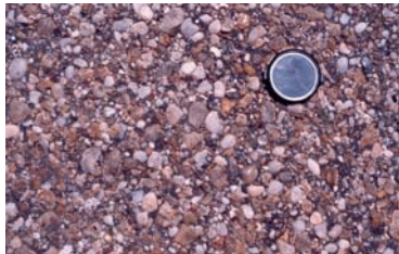
Screened gravel used as surfacing aggregate in the Otta seal.
