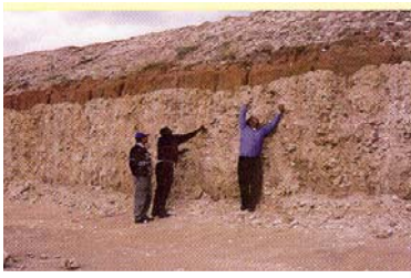
Naturally occurring calcrete found under a thin layer of overburden.
