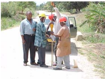
Direct strength measurement with e.g. DCP can assist in calibration of method specifications, but cannot replace material management and continuous and skilful observation of the work procedures as the most powerful means of quality assurance where variable and marginal materials are used.
