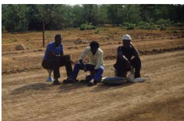
Density control is important in 'calibration' of method specifications, but full scale test programmes are not always viable on LVSRs due to lack of resources.
