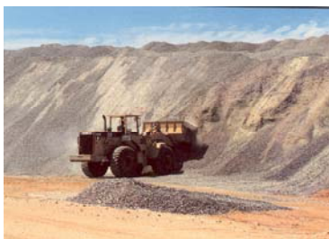
Crushed limestone is a typical "standard" material that is produced by crushing of blasted, massive rock to a defined grading.
