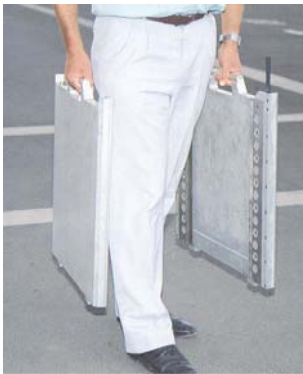
Portable weighbridge system.
