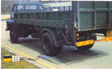
Measurement of rear axle load using portable weighbridge.
