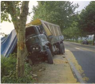
An unforgiving roadside is one which is not free of obstacles that may cause serious injuries to occupants of heavy vehicles
