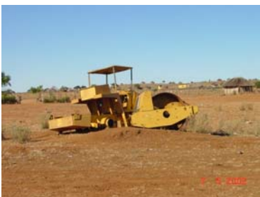
Very often, worn out construction plant is abandoned and becomes an eyesore. The contract documents should cover removal of unwanted plant to an approved area.
