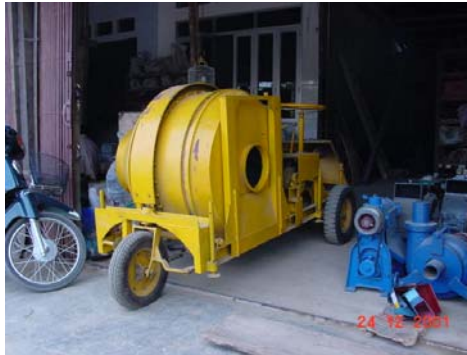
Figure 74: Concrete mixer with capacity of 5m 3 /h
