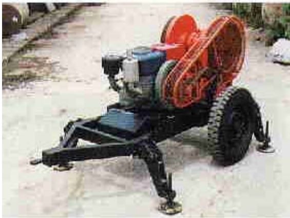
Figure 73: Low capacity stone crusher (5m 3 /h)
