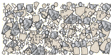
Figure 68: Aggregates of different size mixed together following grading rule to make gravel.
