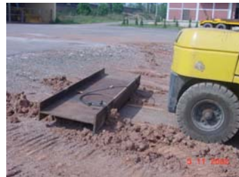
Figure 48 Steel I beam (400mm depth section) drag. Can be surcharged to increase weight if necessary
