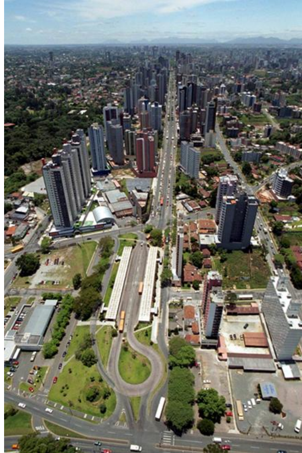
Picture 27: Cities are places where people and activities come together (businesses, universities, museums etc.) which increases accessibility and reduces transport costs. This can be supported by transit-oriented development i.e. high density and mixed land use along transport corridors like in Curitiba (Brazil), cities can move to a low-carbon transport sector.
