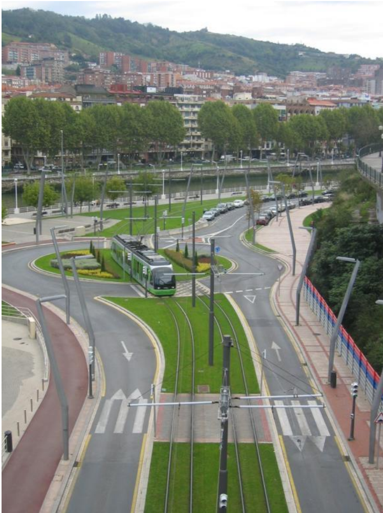
Picture 31: Quality matters! It is not about deciding about policies, it is about ensuring the best possible implementation. High-quality implementation in Bilbao (Spain) shown in this picture, is reflected in human-scale road design (calming of road traffic, separated bicycle lanes, pedestrian crossings), convenient integration of non-motorised traffic and transit and pleasant design.
