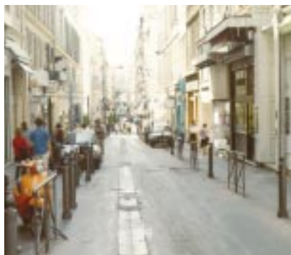
Bollards and gates, separate pedestrians from traffic, enabling a level surface and a greater feeling of pedestrian importance
