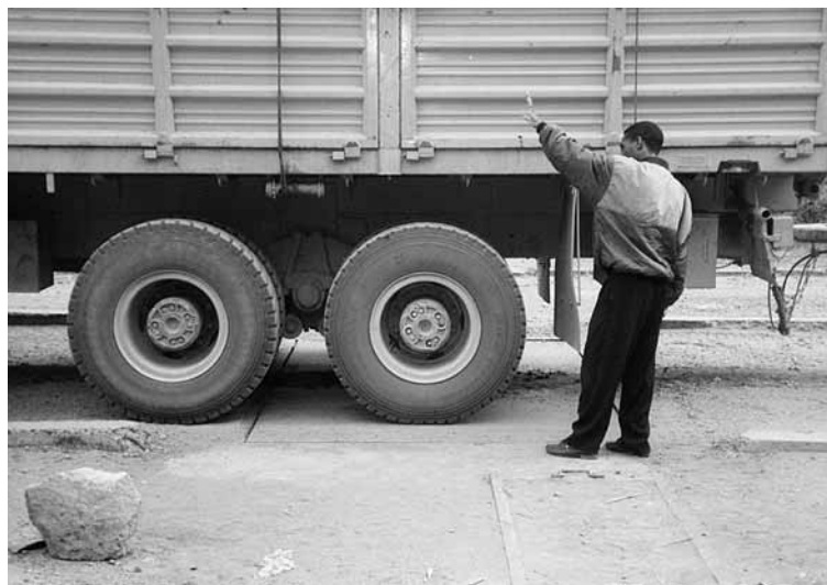
Figure 5b Axle on fixed weighbridge
