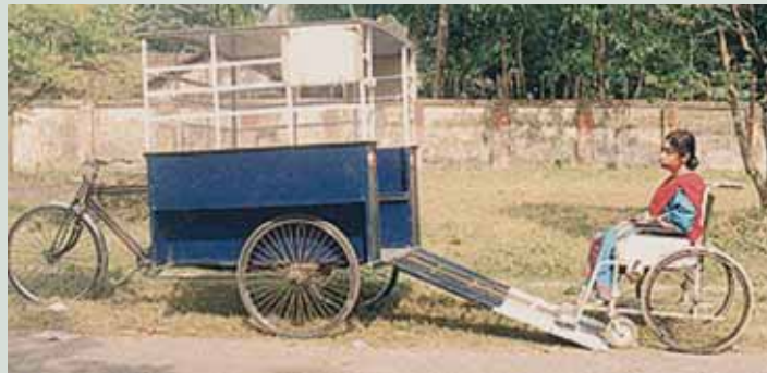
Figure 3.50 Experimentation to the development of this wheelchair accessible bicycle rickshaw. Photo by the Bikash Bharati Welfare Society in India (Courtesy of Lalita Sen)
