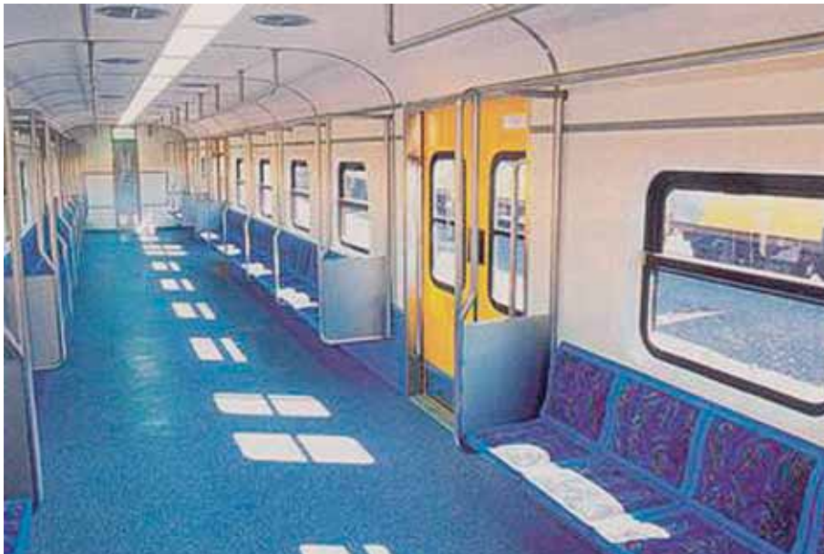
Figure 3.54 An unobstructed train carriage interior with improved colour contrast and grabrails, Cape Town, South Africa ( Source: Charles O’Leary, courtesy of Modalink )
