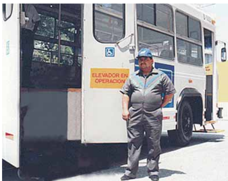
Figure 3.36 This accessible bus in Mexico City features a lift and a retractable front step (Source: AEI)
