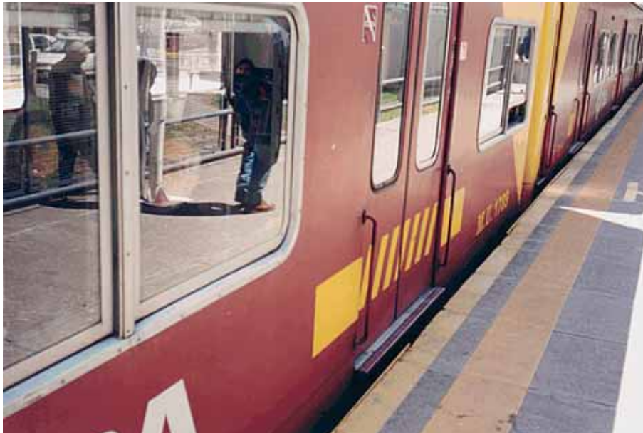
Figure 3.52 (Near) step-free entry into the Buenos Aires railway carriage
