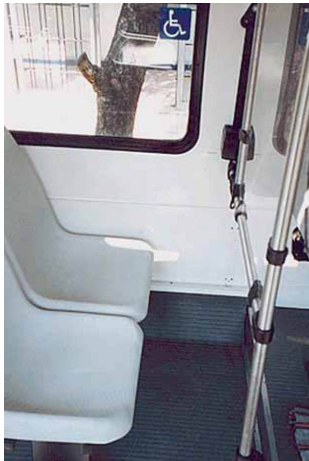
Figure 3.39 Priority seating behind the driver, used in midibuses in Mexico City
