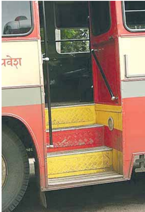
Figure 3.42 Low-cost improvements to this bus entrance included installing extra handrails, colour contrasted steps and lighting
