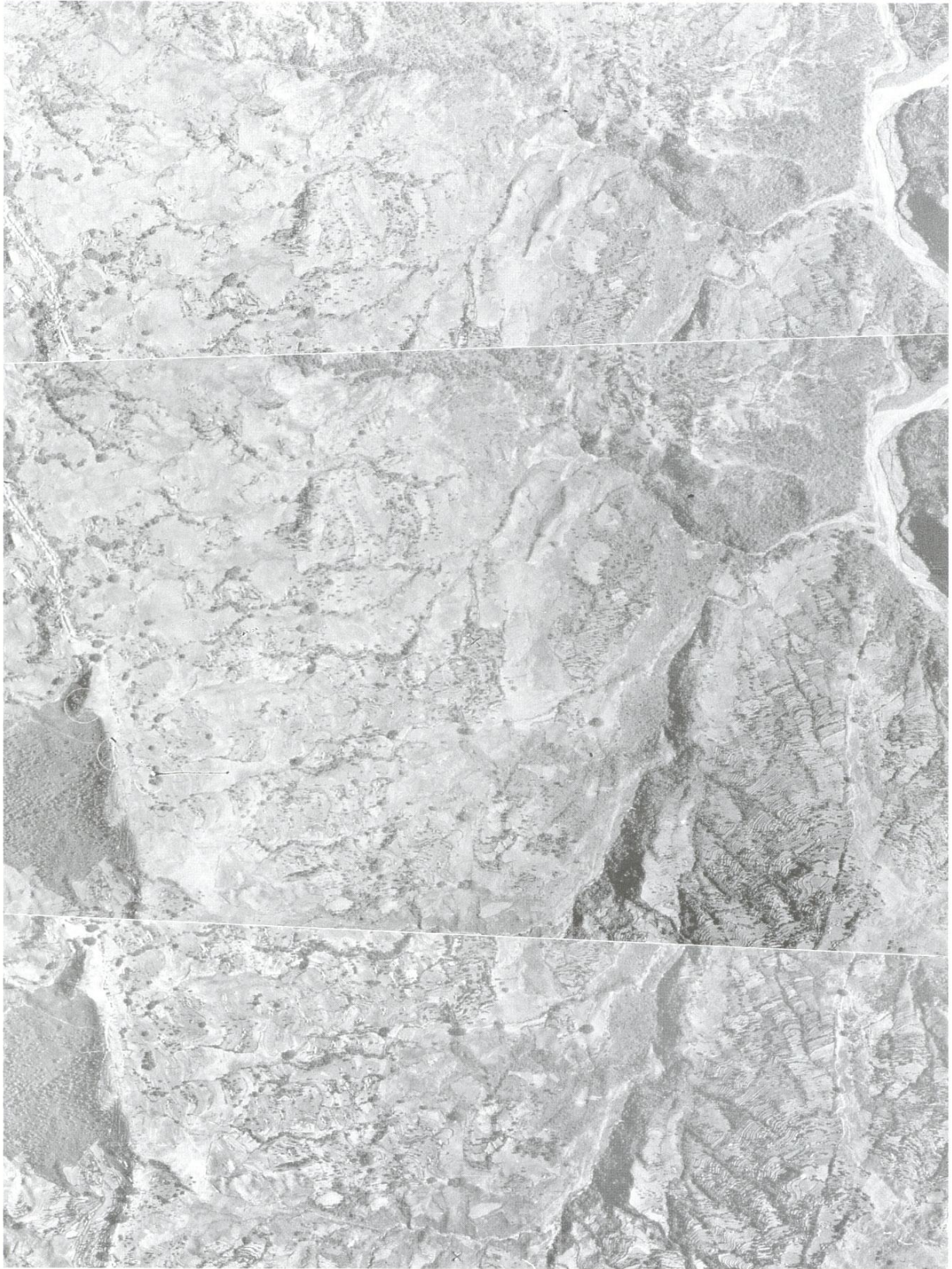
Figure 5.3 Aerial photograph interpretation for road alignment purpose- Stereoscopic pair of aerial photographs
