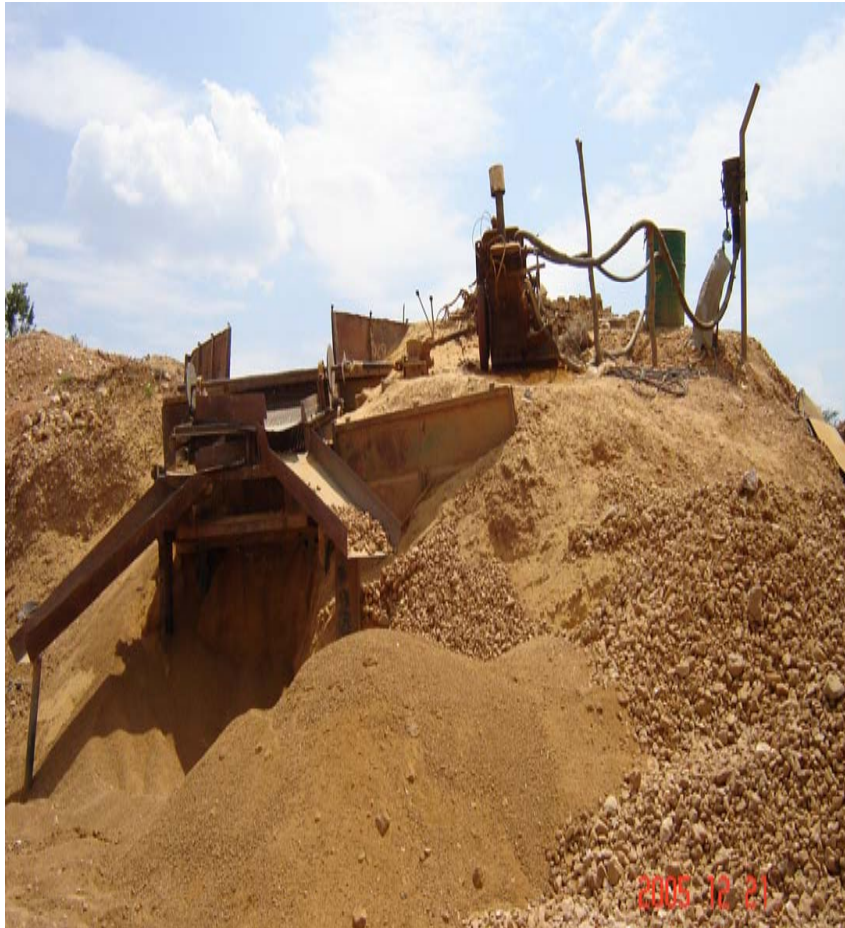
Photo 1 and 2: Small Locally Fabricated Aggregate Screening Plant for Otta Seal Project in Kagera Region (Left) and Chipping Production Plant for Conventional Bituminous Surface Dressing Project in Rukwa Region (Right)
