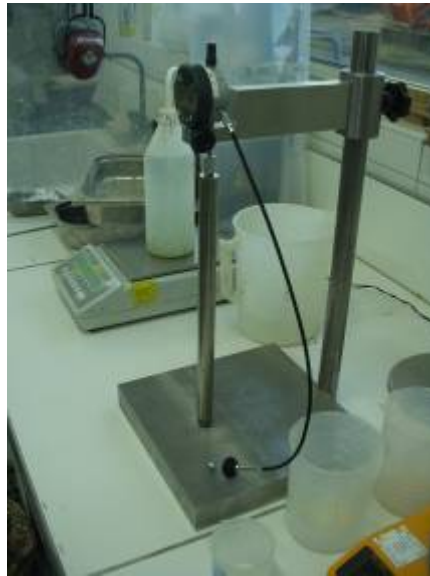
Figure C.2.5: Tool realized for length measurement of Ø16x 32 cm of well graded aggregate. The zero is made thanks an invar bar. The contact with the inserts of the sample or the bar are ensured by two steel balls.
