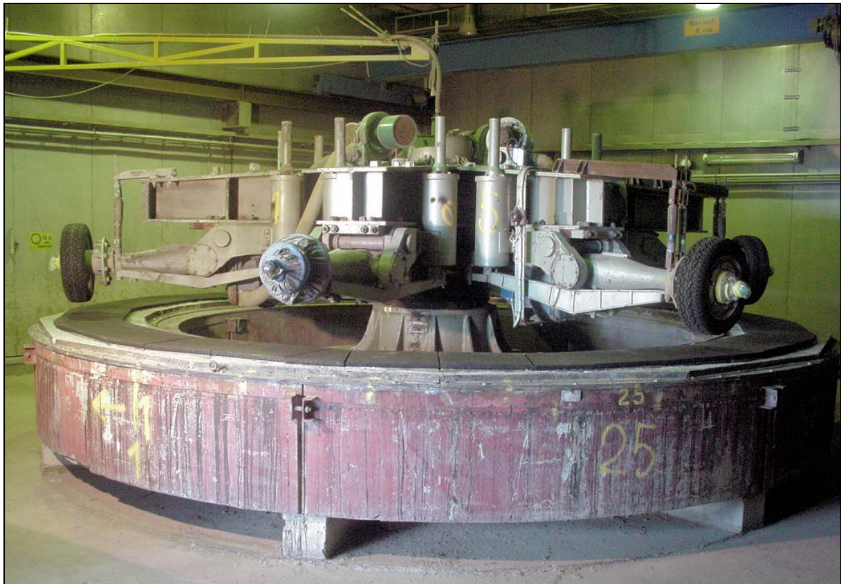
Figure C.5.1: The Pavement Testing Machine at VTI.
