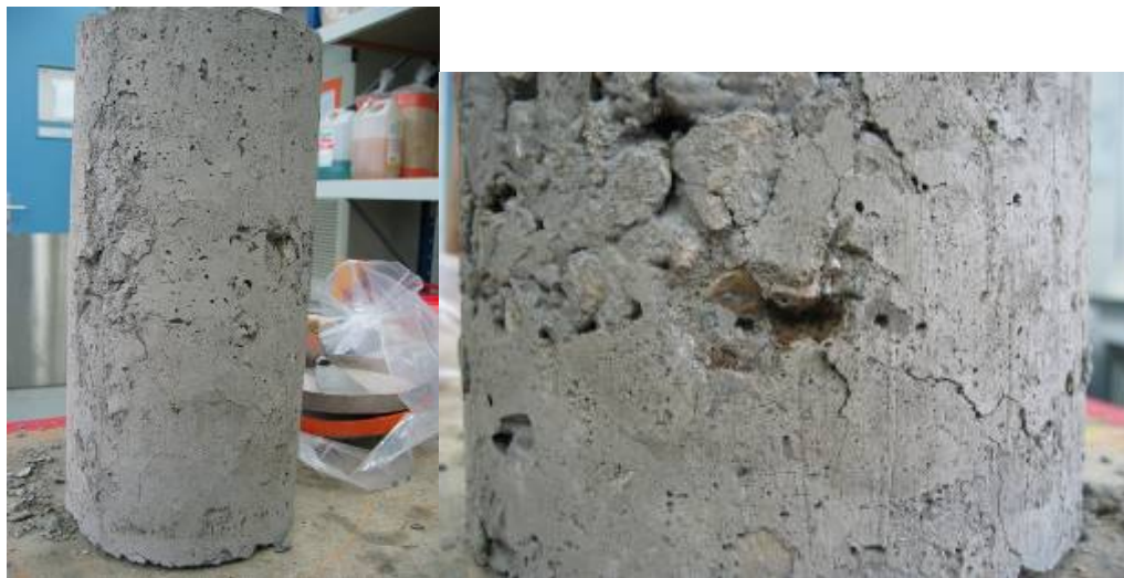
Figure C.2.3: Pictures of the F1 mix after curing. Segregation is due to the gap graded skeleton. Cracks are visible as well as brown scaling due to quicklime hydration in slag particles
