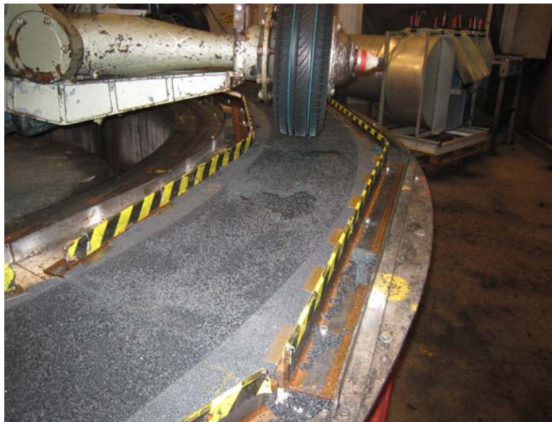
Figure C.5.8 Broken plate at after 23 000 revolutions in the PVM.
