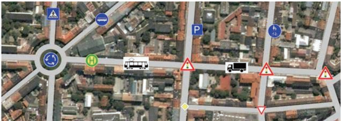
Figure 3.7. Interrupted Flow Facilities
