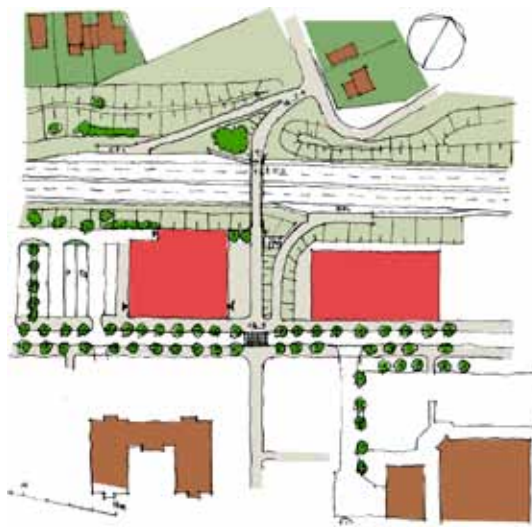
Illustration of the alternative plan for Riksväg 55 at lowered elevation. From Uppsala Workshop – Highway 55, Kvarnbolund–Berthåga section.
