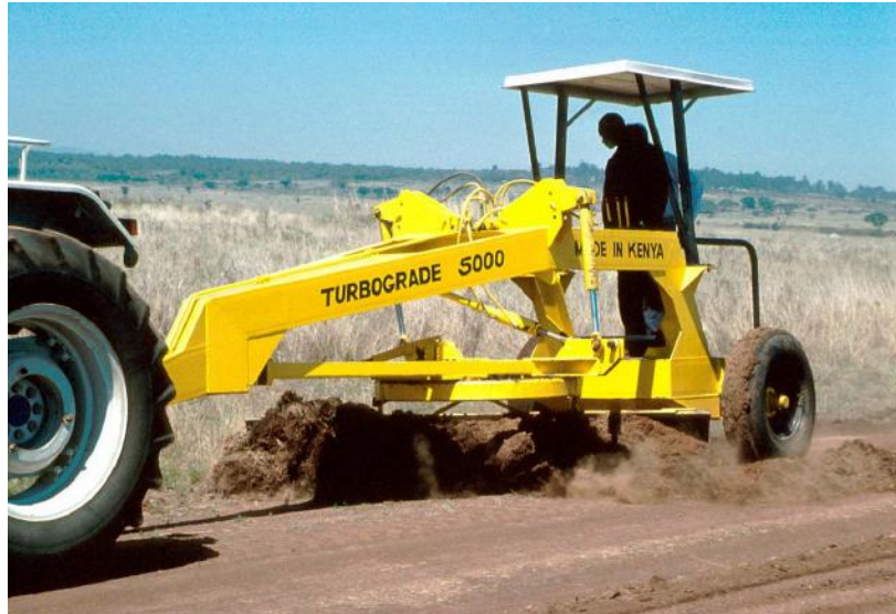
5 tonne heavy towed grader, CMC Motors, made in Kenya
