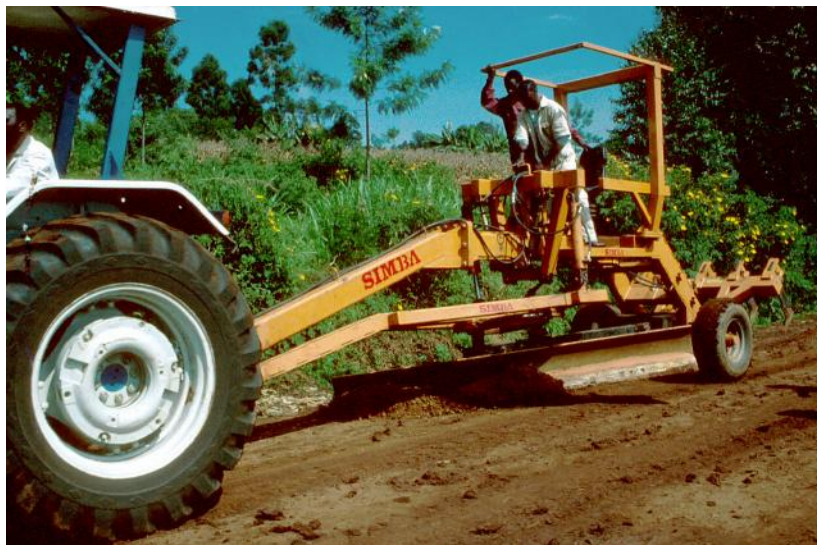
3.5 tonne towed grader, Simba, UK
