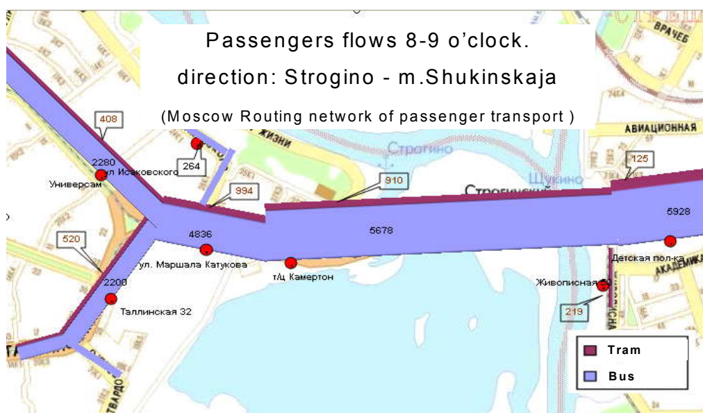
Fig.10 Intensity of passenger's flows along the arterial roads and main multi-modal intersections (example of the analysis)
