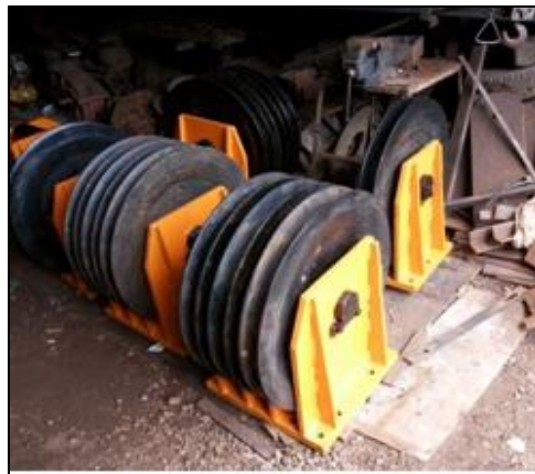
FIGURE 8 3-Sheave pulley blocks
