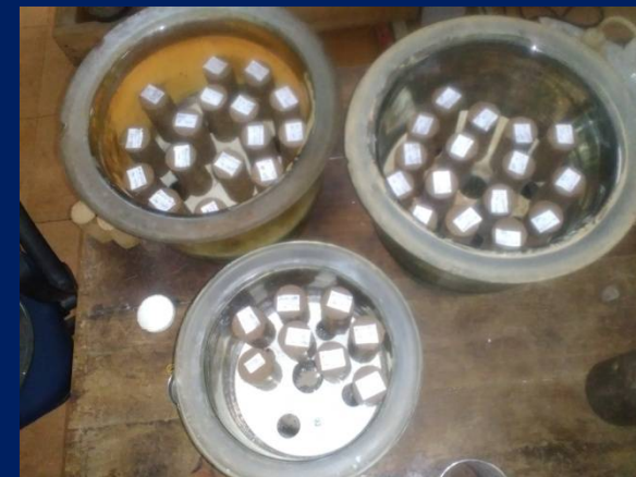
Curing of UCS samples in dessicator
