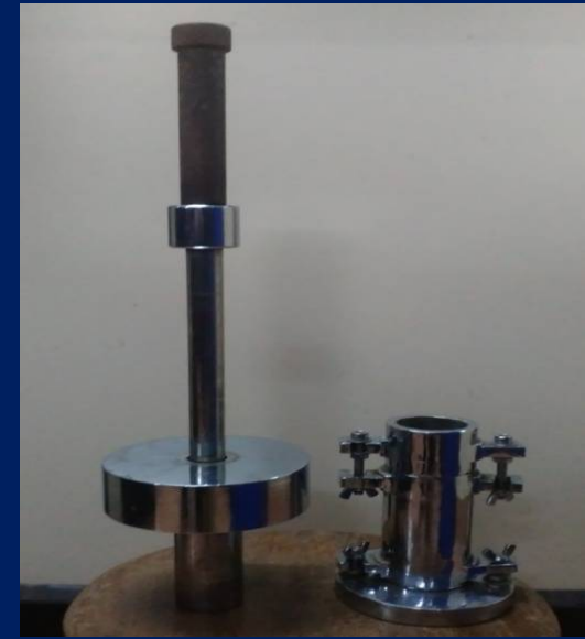
Miniature compaction and CBR mould, Patent file no. 201621013680 , Kulkarni, Dutta and Mandal (2016)
