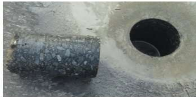
(C) Fresh Core Extracted from Bituminous Layers
