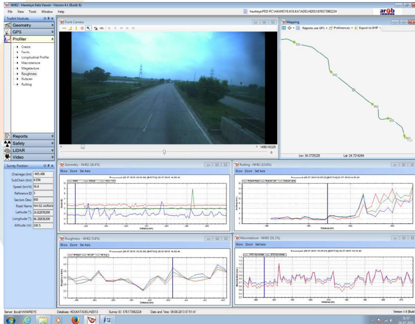
A View of Road Information System showing all Data along with GIS Map and Right-of Way Images
