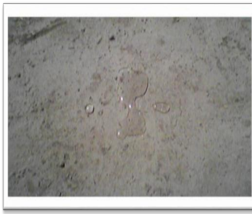
Water Drop Test
