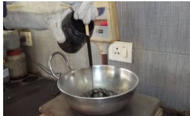
IMAGE 2 adding cold mix binder as per gradation
