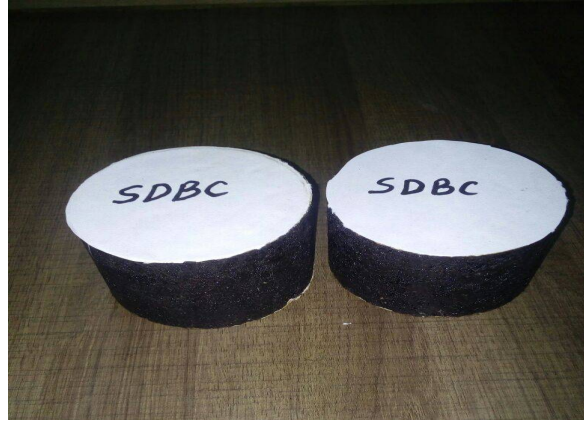
IMAGE 7 mould of cold mix SDBC prepared for Marshall test
