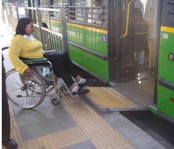
FIGURE 2 Higher bus stop platform and lower bus chassis
