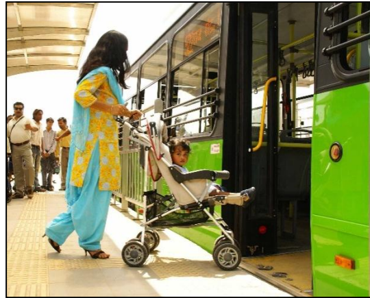
FIGURE 11 LFB floor heights synchronized with the platform height to achieve level access
