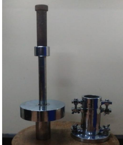
FIGURE 2 Miniature CBR apparatus [22]
