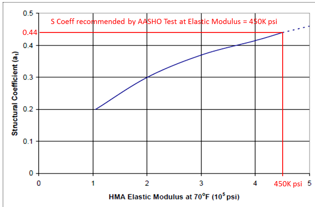
CHART 1.0 Structural Coefficient Vs. HMA Elastic Modulus
