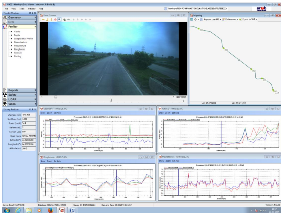
FIGURE 3 A View of Road Information System showing all Data along with GIS Map and Right-of Way Images
