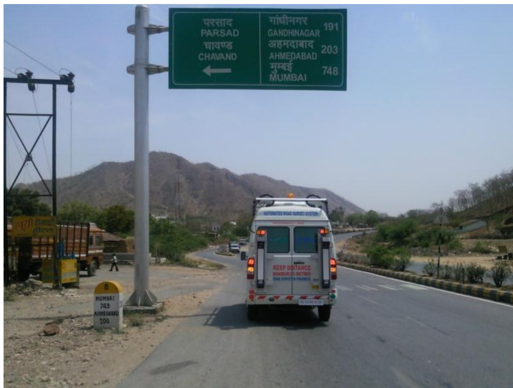
PHOTO 1 Measurement of Road Inventory and Pavement Condition Using Automated Road Survey System on NH-08
