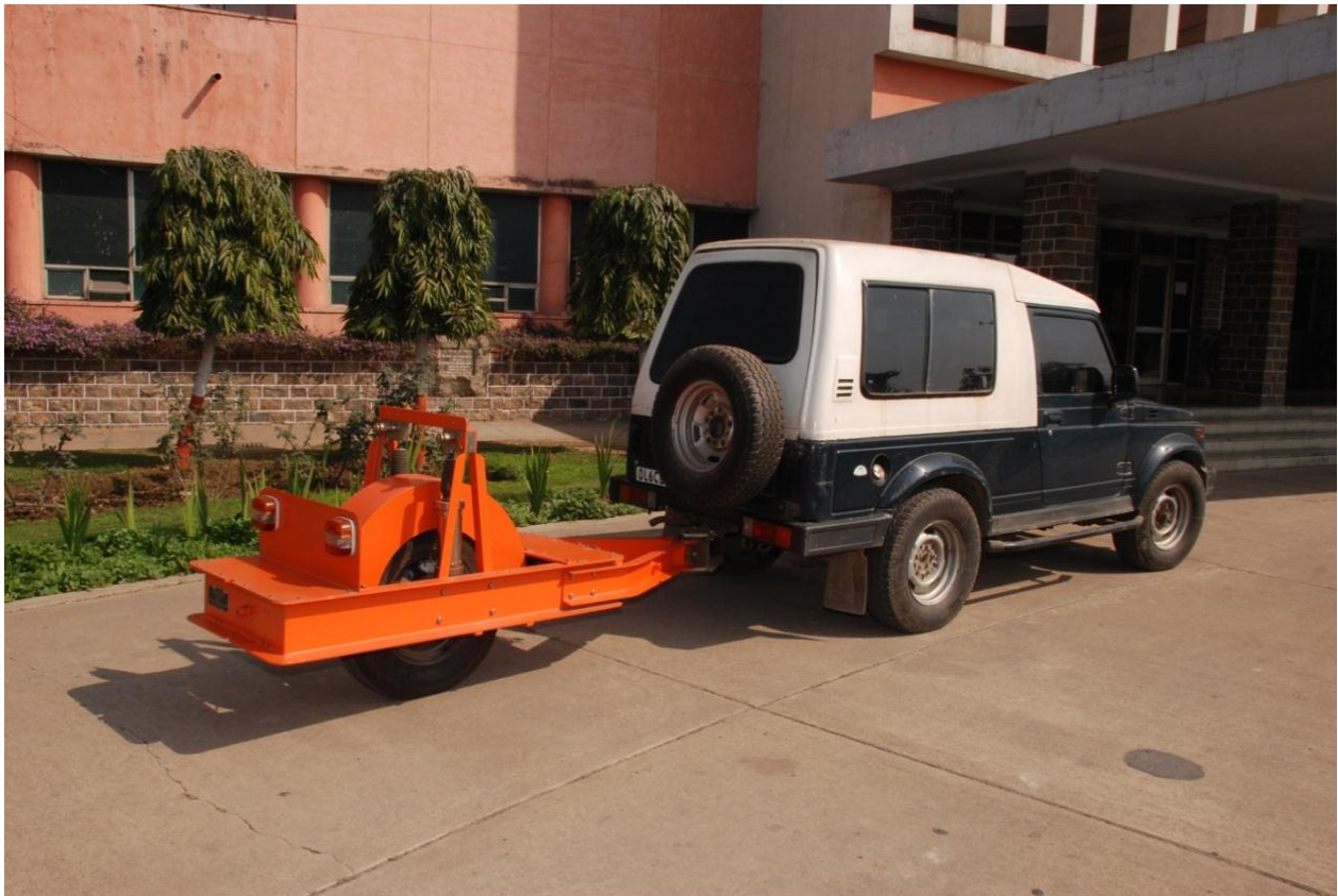
FIGURE 1 Automatic Road Unevenness Recorder (ARUR)
