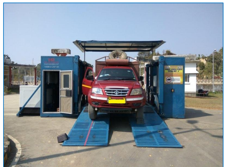
Figure 3- Mobile Inspection Lane at NATRiP Silchar center
