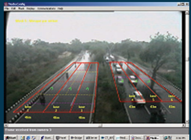
Figure 1: Lane configuration of the Video Incident Detection System
