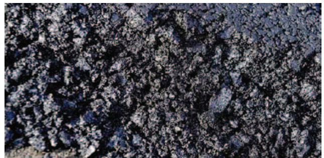
Low-temperature asphalt with foamed bitumen can be installed at around 110 °C with no compromise in quality.
