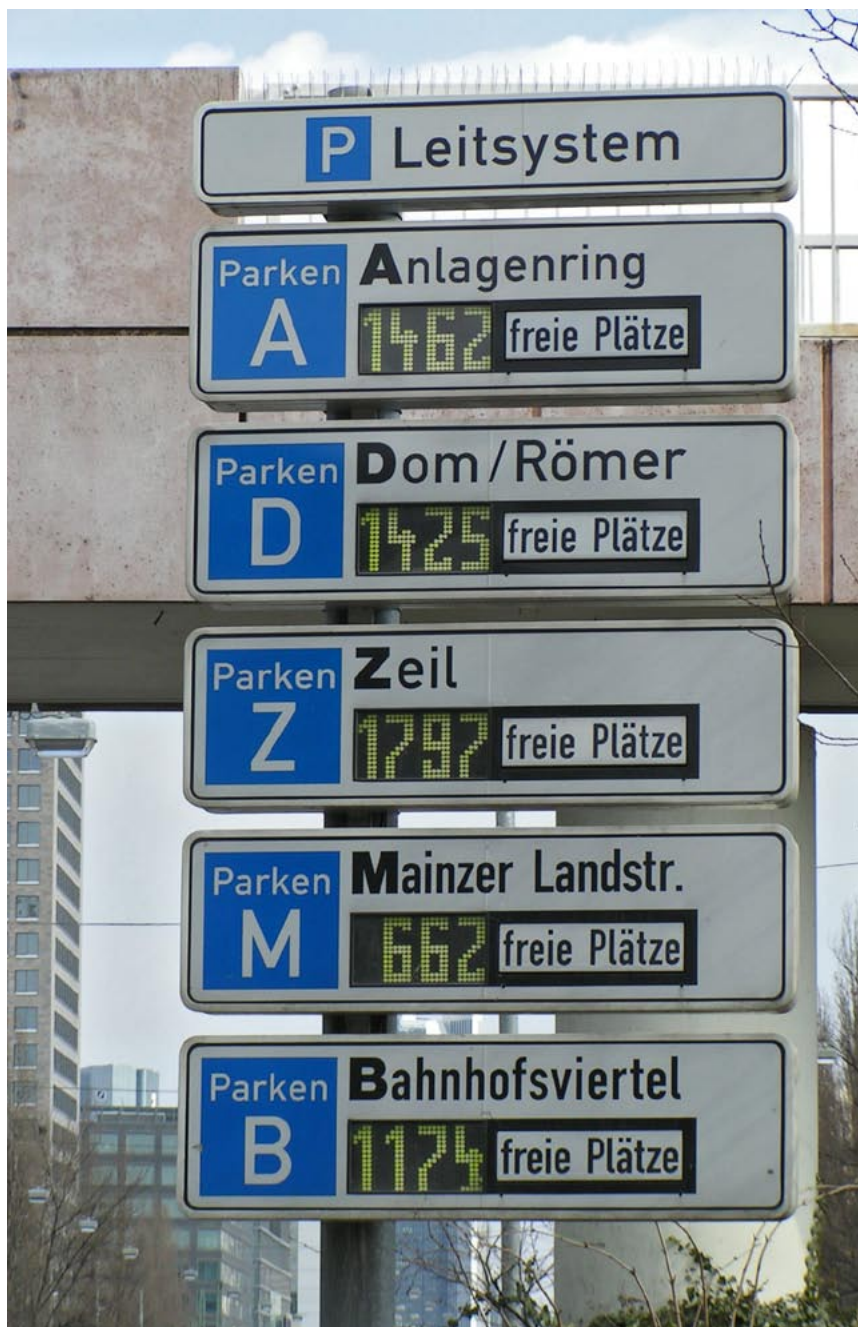
Figure 19 This sign is part of a city-wide parking guidance system and provides information on available space in car parks.
