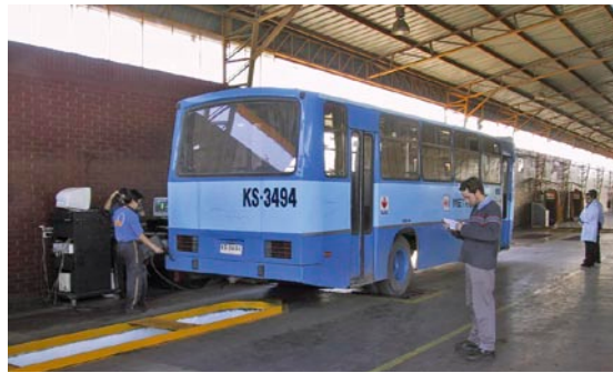
Fig. 21 Exhaust emission laboratory, Centro de Control y Certificación Vehicular. This facility carries out type approval testing for new vehicles. Frank Dursbeck
