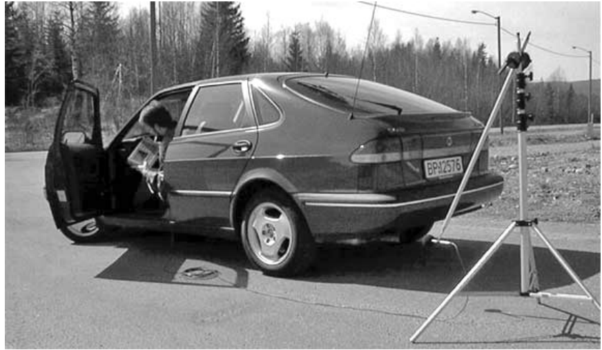
Fig. 34 Sound level measuring installation. Norsonic
