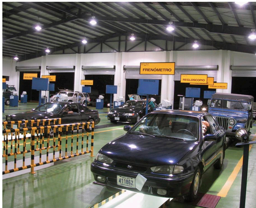
Fig. 29 Test station with six inspection lanes in Heredia.
