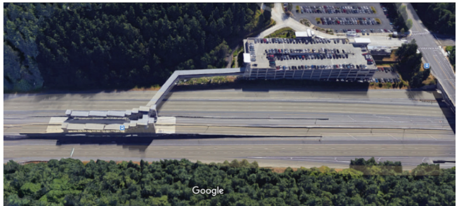
Mountlake Terrace Transit Center, showing causeway to freeway median (top) and freeway median station (bottom).
