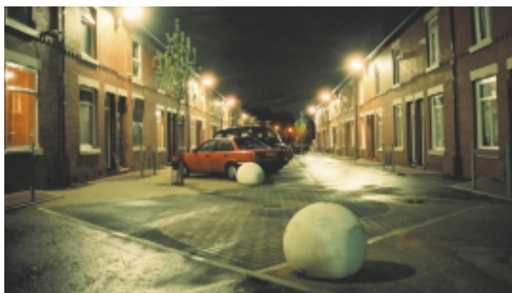
Well-designed lighting at Northmoor gives high levels of illumination during the evening, but reduces in intensity after midnight, see Case Study 9.
