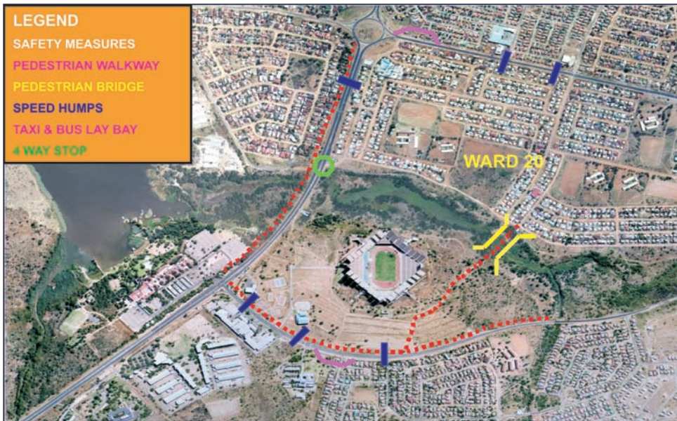
Aerial photograph showing proposed road safety measures
