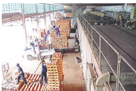
Bricks are burnt inside a tunnel on a railbased production line.
