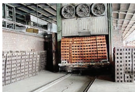
Bricks are burnt inside a tunnel on a railbased production line.
