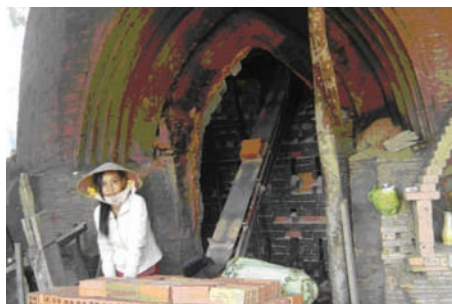
Unloading fired bricks through the kiln entrance with the aid of an electric powered conveyor. (Note that the hollow bricks shown are not suitable for road paving).
