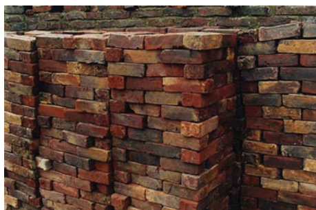
Burnt clay bricks stacked ready for use.
