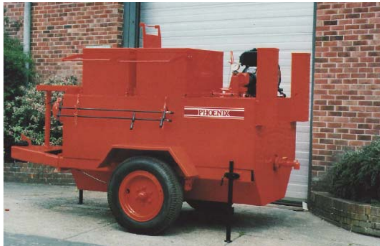
Figure 32: Towed bitumen heater-distributor
