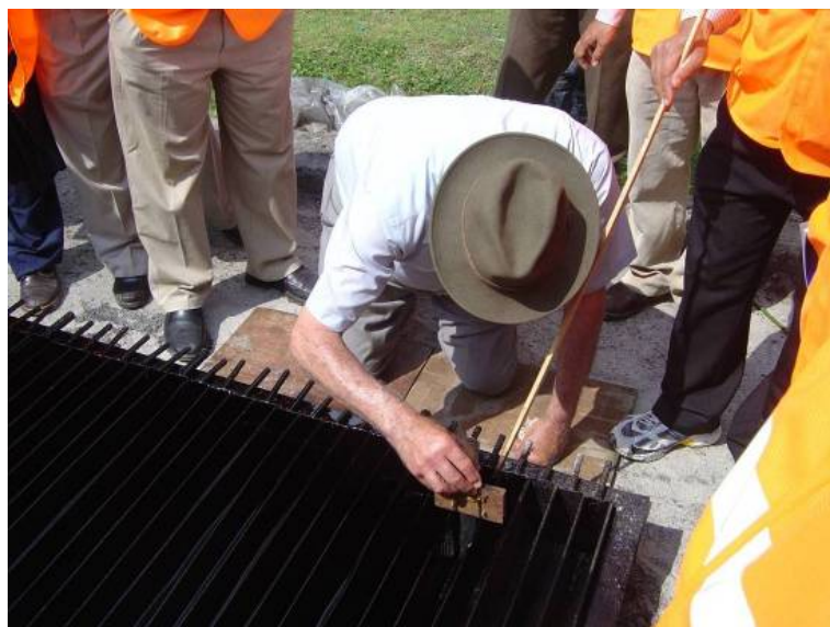
Figure 15: Measuring the bitumen in each tray
