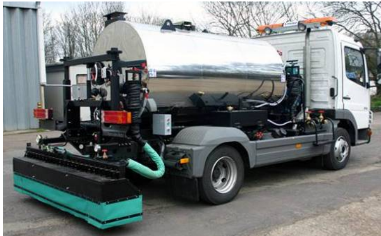
Figure 21: A bitumen distributor using swirling nozzles
