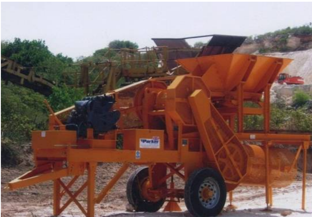
Frame No: 002 Description: Mobile Crushing Plant
