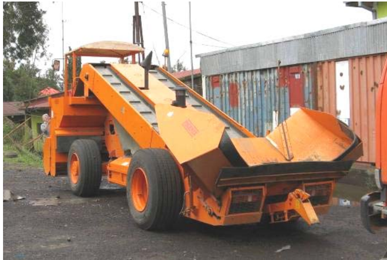
Figure 29: Self-propelled chipping spreader
