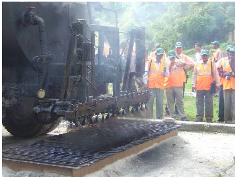
Figure 13: Depot Tray test in Nepal
