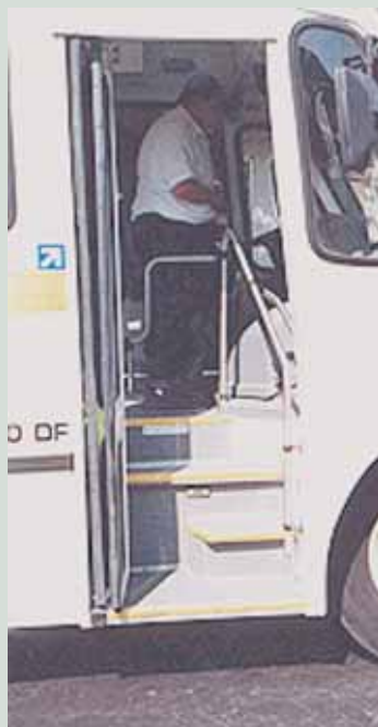
Figure 3.34 Concession agreements can require low-cost features such as contrasting steps and handrails on midibuses
