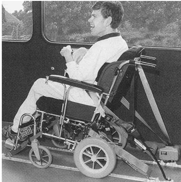
Figure 3.41 The wheelchair and passenger are both restrained in a vehicle using a 4-point restraint ( Source: Unwin Safety Systems )
