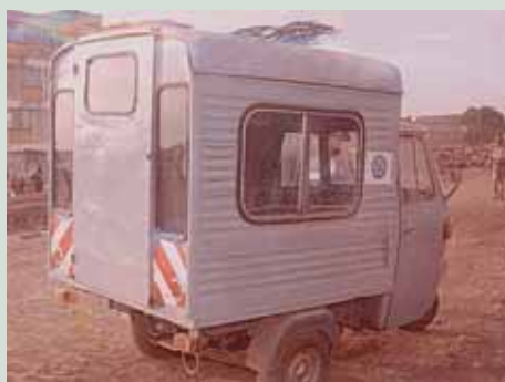
Figure 3.51 Side and rear view of a 3-wheeled motorcycle turned into a prototype accessible van (Courtesy of Wycliffe Kepha)
