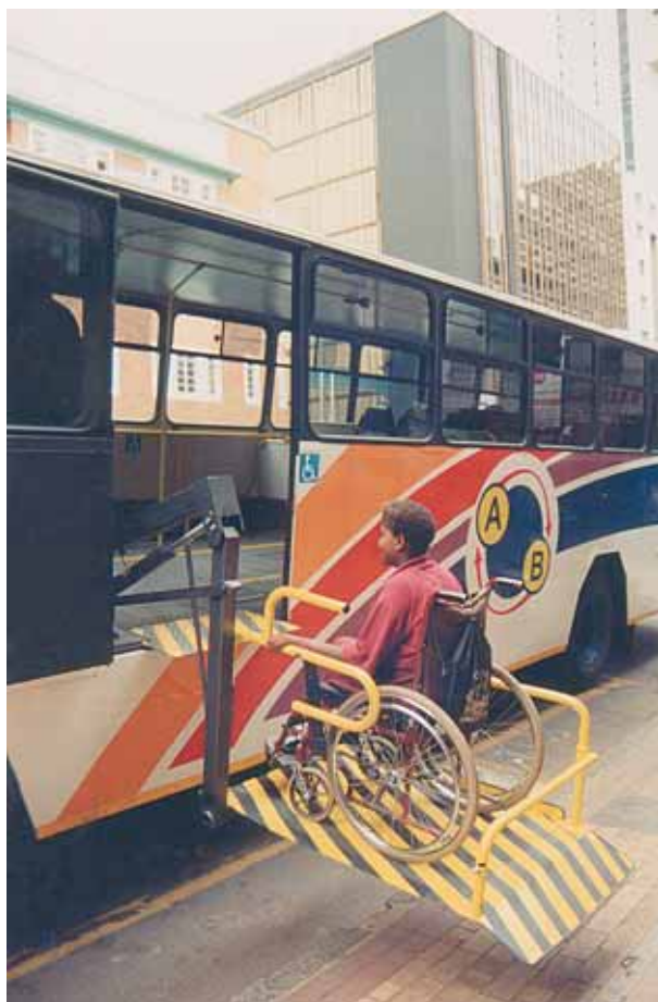
Figure 3.40 A slide-door wheelchair lift in use in Pretoria, South Africa (Source: CSIR)
