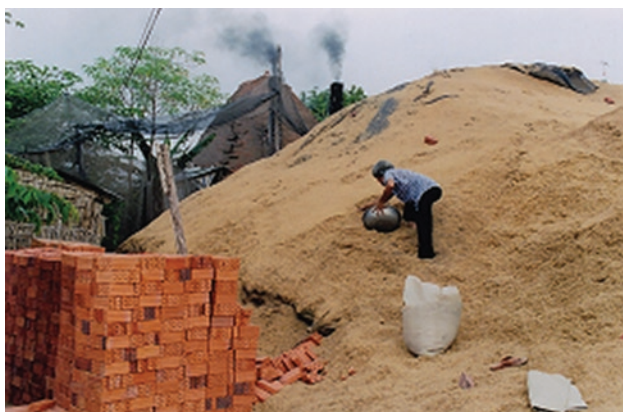
Photo 7: Clay Brick production using rice husk fuel
